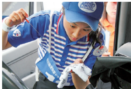
Engine oil inspection
